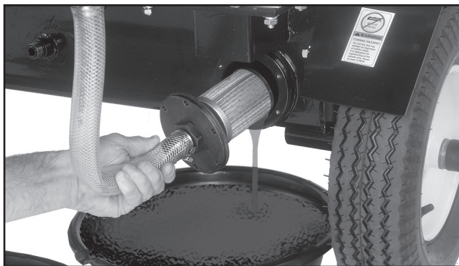
Figure 24. Draining hydraulic fluid.
